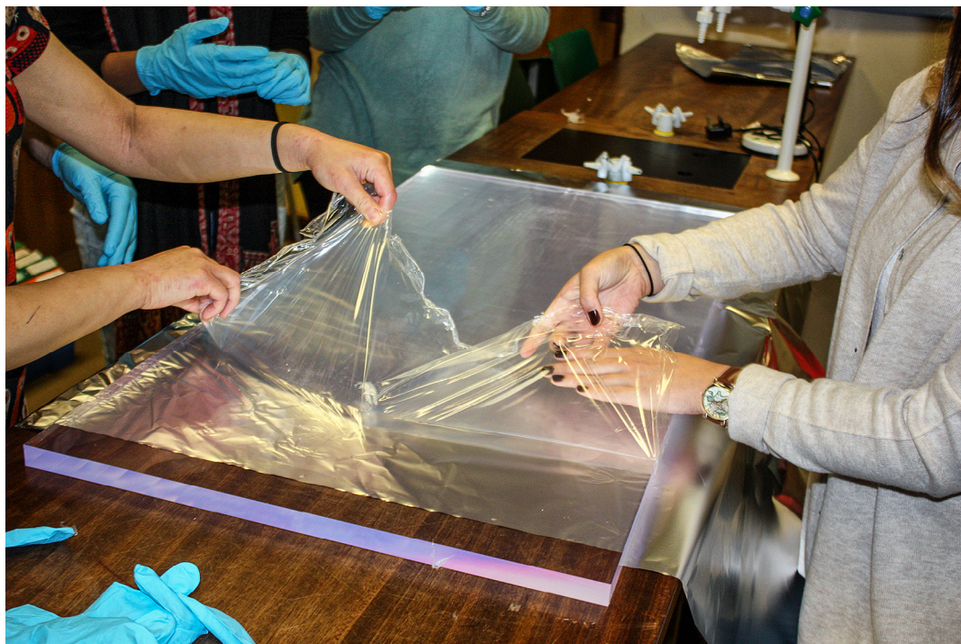
Figure 3 Sixth-form physics students (age 16–17 years) preparing the scintillator for the detector
